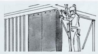
Measure the length to be applied and then cut a similar length of AstroShield, adding an inch or two to assure complete coverage at top and bottom. At corners, wrap around the corner and continue vertical installation. Cut a second length and position next to the first length. Butt sides evenly together or slightly overlap. Tape all seams.
