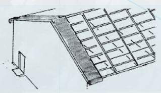
Starting at the end of the roofing framework, measure the length across the trusses, adding enough to allow hang at both ends. Cut the first piece and lay in place. Pull tight from both ends and attach to trusses and purlins using self-tapping screws and washers or with pressure-sensitive reflective tape. Cut the second length, laying parallel to first. Make sure to butt or slightly overlap edges. Tape all seams.
